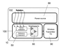
be fabricated using CMOS processes, which facilitates integration of the radiation sensor with signal processing and transceiver electronics. A wireless transceiver can be integrated with the dosimeter to enable remote activation and reading of the sensed radiation value.
